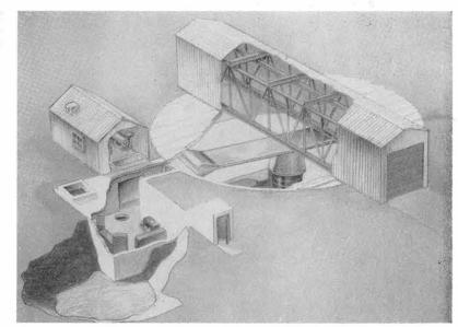
NEW CENTRIFUGE, largest in the free world in terms of dynamic load capacity, is being built for Sandia Laboratory. Installation will be adjacent to the present centrifuge in Area III. The new facility will be used to simulate vibration and acceleration of rocket launch and reentry.
